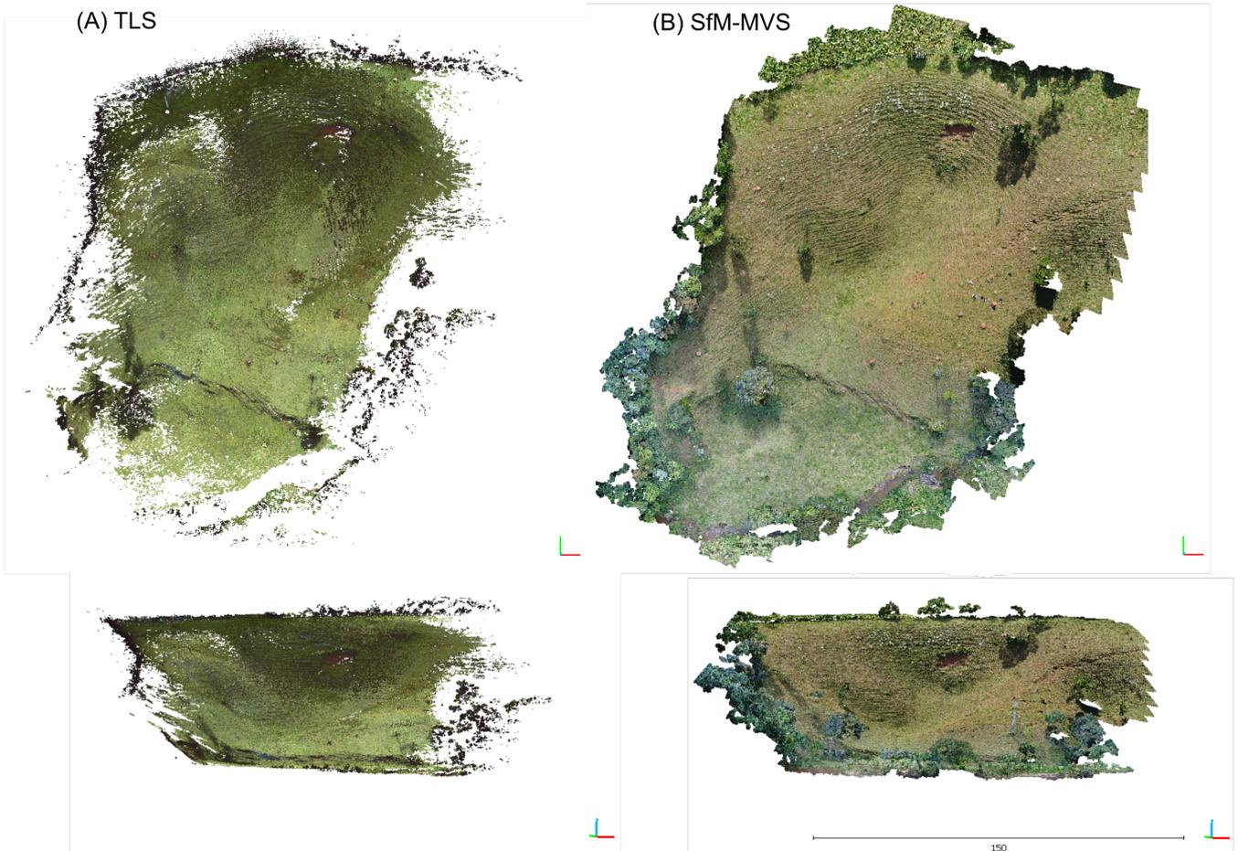
Figure 2: TLS (A) and SfM-MVS (B) point clouds.
